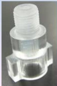
The flow straightener we designed has a replaceable core made of glass micropipettes that can be removed completely for unrestricted flow.
